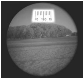
Figure 2-12. View Through Installed Compass
