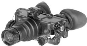
Figure 2-6. Installation of the IR Spot/Flood Lens
