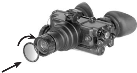
Figure 2-5. Installation of the Light Interference Filter
